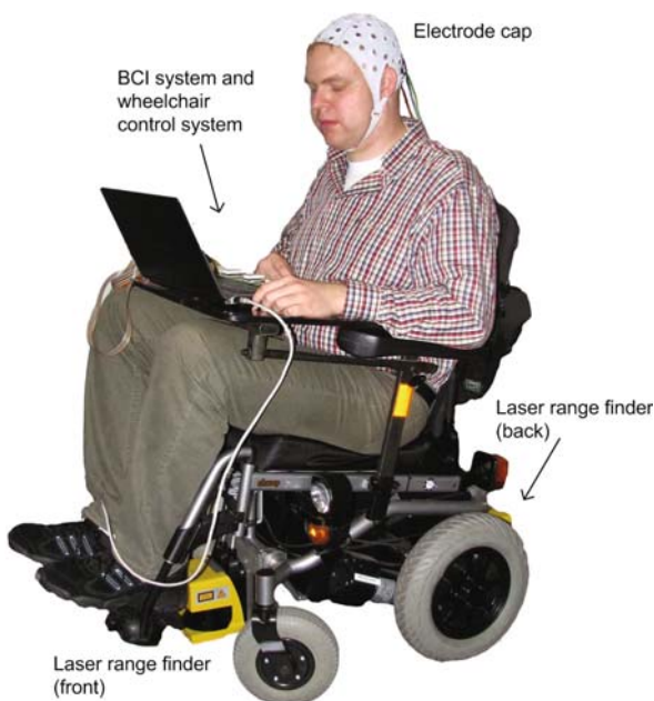
Fig. 6.7 Bremen autonomous wheelchair Rolland III controlled by the Bremen BCI
